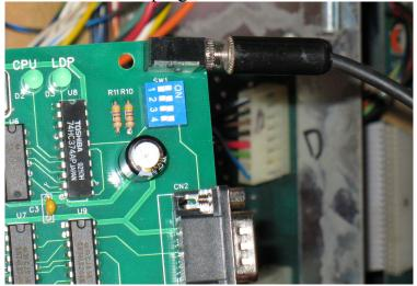
Connect the serial Interface cable from the player to LaserCon's CN2.
